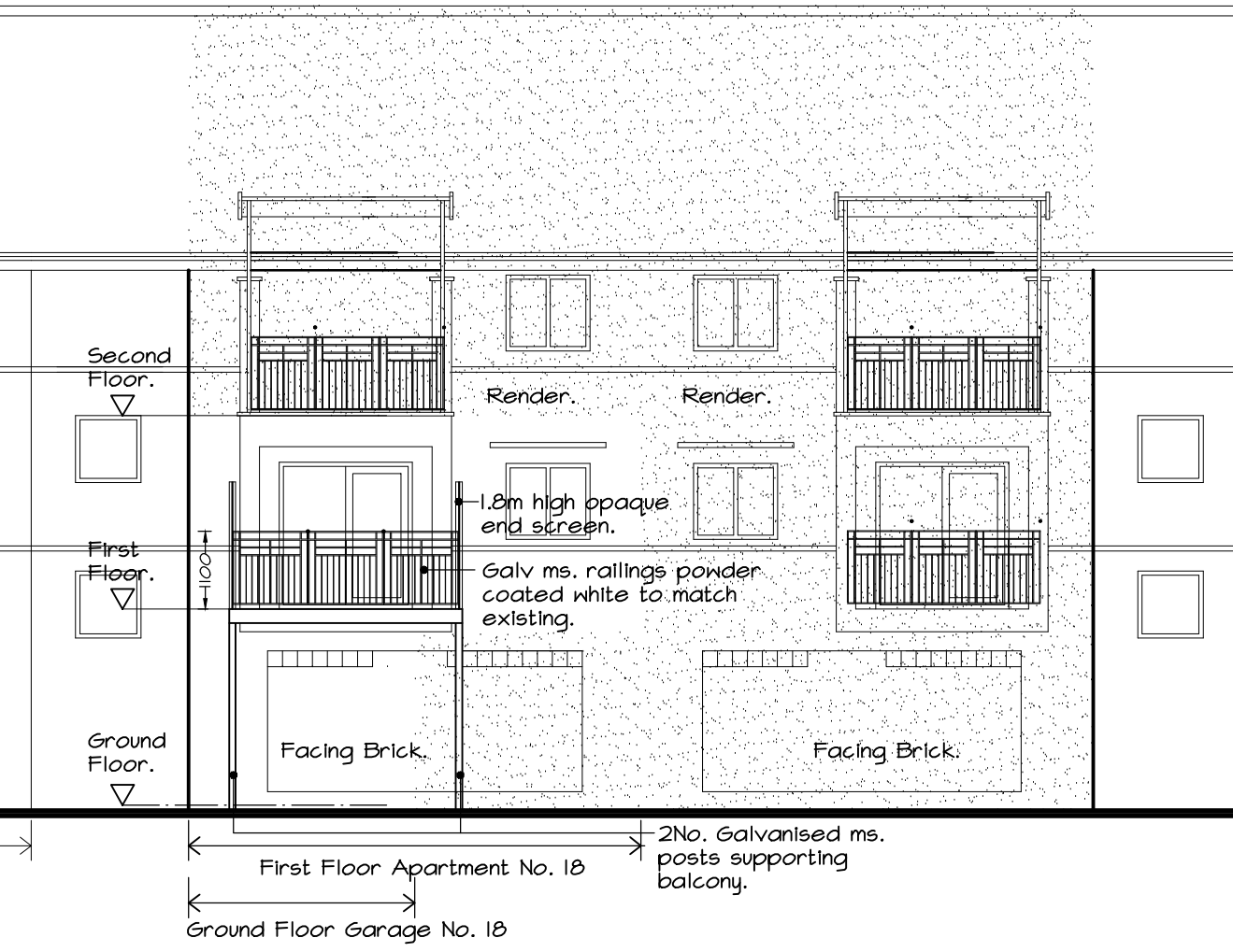
SOUTH WEST ELEVATION.
